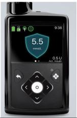
This pump can be used as a normal pump but also has an additional programme called Smart Guard which can be used with the Guardian continuous glucose monitor. Smartguard technology automatically adjusts insulin delivery based on sensor glucose readings and autocorrects. ump is connected to the body with a cannula and tube.
